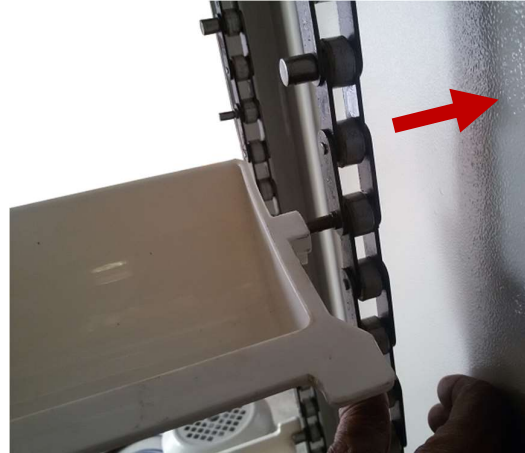
Placing bucket on the right side chain by pushing the chain to right side
